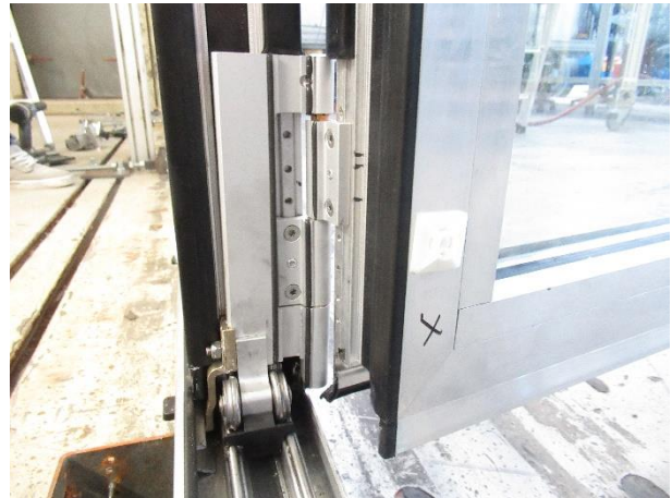
Picture 16 Door hinge main sash, seen from rebate
