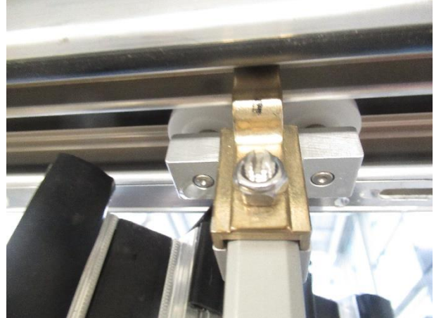
Picture 10 Top guide roller, seen from side
